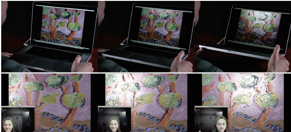
Fig. 8. Image sequence showing a painting model being displayed on the tangiBook. The tangiBook is based on an off-the-shelf laptop computer that incorporates an accelerometer and a webcam as standard equipment. Custom software allows the orientation of the laptop screen and the position of the observer to be tracked in real-time. Tilting the laptop (as shown) or moving in front of the screen produces realistic changes in surface lighting and material appearance.
